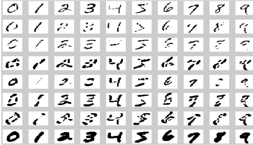
Figure 4: Tangent vector: The first row shows the original images and other rows are different tangent vectors from different transformation. Starting from the second row, each transformation is: x-translation, y-translation, rotation, scaling, parallel hyperbolic transformation, diagonal hyperbolic transformation and thickness.
