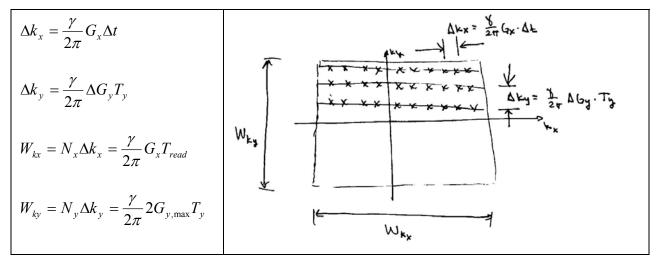
**Sampling in k-space (spatial frequency domain).** Previously we discussed sampling of the object and its effect on the spectrum. Here we have the reverse – sampling in Fourier domain and its effect on the reconstructed object. Again, we will perform our sampling by multiplying a function times the 2D comb function. With sample spacing of  $\Delta k_x$  and  $\Delta k_y$ , in the  $k_x$  and  $k_y$  directions, the sampled Fourier data is:
