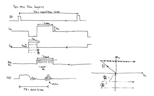
This is a repeated pulse sequence with a different y-gradient value for each RF excitation (TR interval). Let's look at the x-gradient – as in the case of 1D imaging, above, this gradient encodes the *x* spatial position into frequency. This is often called the "frequency encoding" gradient or *x*, in this case, is known as the "frequency direction."
