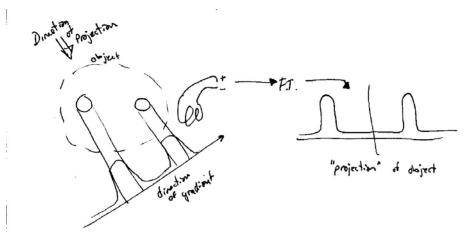
We'll discuss (in the section on computed tomography) the methods for reconstructing images from 1D projections. For now, suffice it to say that if we acquire enough projections, we can fully determine the underlying object. The pulse sequence used by Lauterbur is given here:
