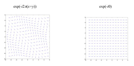
In MRI, the integration is performed by the integration of voltages in the RF coil. The phase variation is performed by the gradients – by shifting the field (and thus frequency) in a spatially linear fashion for a period of time, the magnetization will rotate to a new orientation (in the complex plane). Thus MRI has exactly the same mechanisms as the FT operation.
