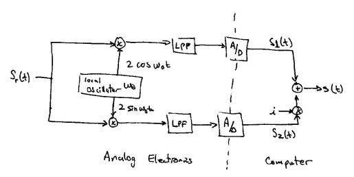
We first look at the upper and lower channels of the complex demodulator for a single component of the received signal at location **r**. The upper channel of the demodulator yields:
