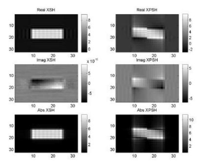
In this case the fftshift moves the shift discontinuity to the center of the image. The most common mistake made in this part was implementation of the fftshift on the 1D data vs. the 2D data (the correct approach).
