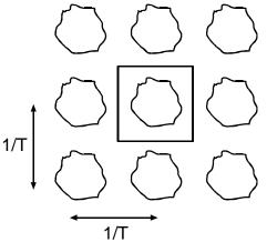
The conditions to prevent aliasing are that the original spectrum, X(u,v), must be bandlimited to the region  $|u| < \frac{1}{2T}$  and  $|v| < \frac{1}{2T}$ , corresponding to the square in the above figure.
