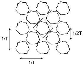
The conditions to prevent aliasing are that the original spectrum, X(u,v), must be bandlimited to the region  $|u+v| < \frac{1}{2\sqrt{2}T}$  and  $|u-v| < \frac{1}{2\sqrt{2}T}$ , corresponding to the square in the above figure. For a circular spectral pattern (which would is typical in optical telescopy), the maximum spectral pattern is reduced by  $1/\sqrt{2}$ .
