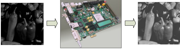
Figure 9. FPGA setup for emulating image-processing tasks, in this case, gamma correction.
