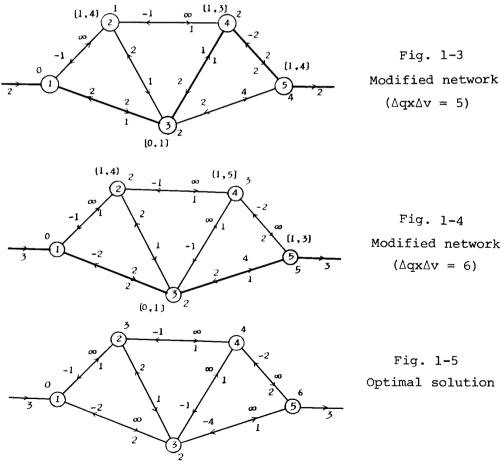
It should be noted that we always have  $\widetilde{d}_{ij}^* \geq 0$  during the course of solution. Since we cannot increase the flow in Figure 1-5, the optimal solution is given by it and the total cost equals  $4 \cdot 1 + 5 \cdot 1 + 6 \cdot 1 = 15$ .
