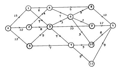
Fig. 2-16 Optimal flow configuration
