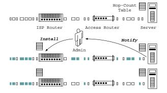
Figure 16: Packet filtering at a router to protect bandwidth.
