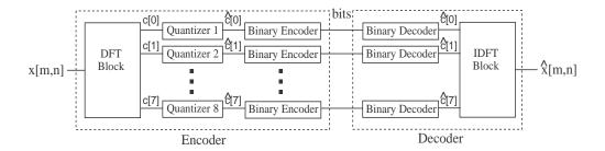
Figure 5.6: A block diagram of a transform coder. The encoder divides the incoming image, x[m,n] into  $1\times 8$  blocks and transforms each block into a sequence of 8 coefficients  $c[0],\ldots,c[7]$ . These coefficients are then quantized to yield  $\widehat{c}[0],\ldots,\widehat{c}[7]$ , and encoded into a binary representation. The decoder creates a reconstruction of the image,  $\widehat{x}[m,n]$  by decoding the binary codewords and inverting the transformation.
