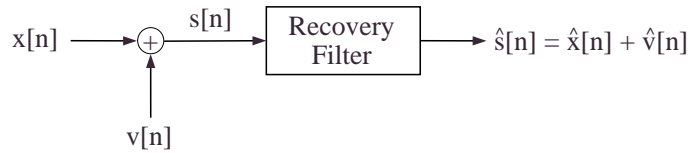
Figure 6.2: A block diagram of additive noise and a recovery filter that attempts to remove the noise.
