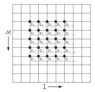
Figure 6.4: The coefficients of a two-dimensional moving average filter. In this figure, pixels exist at the intersection of the horizontal and vertical lines.
