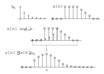
Figure 6.1: A graphical illustration of filtering. The filter coefficients,  $b_k$  and signal to be filtered, x[n], are shown on the top axis. The middle axis shows x[n] and a time-reversed and shifted version of  $b_k$ . We multiply these two signals and sum the result to yield a single sample of the output, y[n], which is shown on the bottom axis. For example, to compute the y[6] sample, we multiply the samples of x[n] by  $b_{6-n}$  and sum the result.
