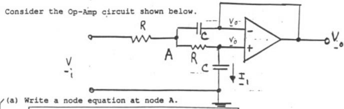
$\frac{\underline{V_A} - \underline{V_i}}{R} + (\underline{V_A} - \underline{V_0}) sc + (\underline{V_A} - \underline{V_0}) = 0$  (1)
