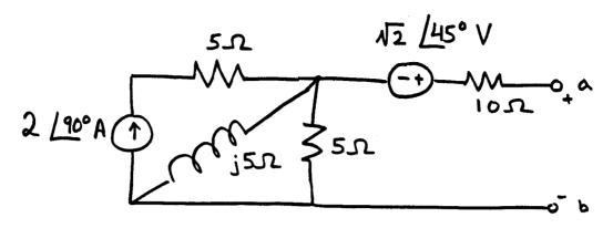
4.a (10 pts) Find the Thevenin equivalent voltage  $V_{th}$  and impedance  $Z_{th}$ .
