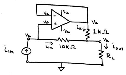
5.a (10 pts) Find the output current  $i_{out}$  in terms of the input current  $i_{in}$  assuming the op-amp is not in saturation.
