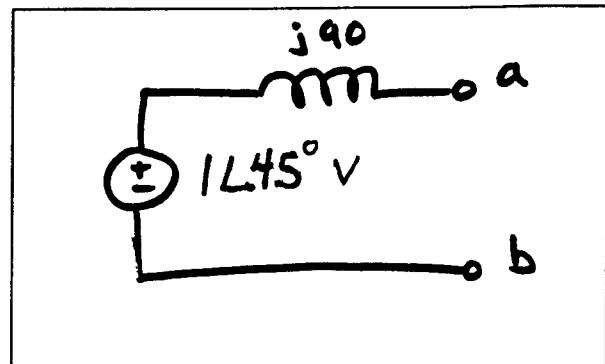
5.b (8 pts) Consider the circuit below. Find the Thevenin equivalent voltage  $V_{th}$  and Thevenin impedance  $Z_{th}$ . Draw the Thevenin equivalent circuit.
