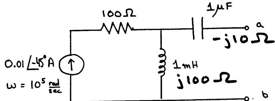
$$V_{th} = V_{ab}^{oc} = (0.01 \angle -45^\circ)(j100) = 1 \angle +45^\circ$$
