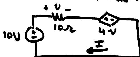
$$-10 + 5v = 0, \quad v = IR = 10I \\ \Rightarrow I = \frac{10}{5} = 2A. \quad \therefore Z_{th} = \frac{10}{2} = 5\Omega$$
