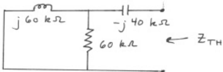
$$\begin{aligned} Z_{TH} &= \frac{1}{j\omega c} + \frac{60(j60)}{60+j60} = -j40 + 30 + j30 \text{ k}\Omega \\ &= 30 - j10 \text{ k}\Omega \end{aligned}$$
