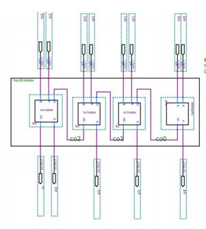
If the verilog file for the adder were to make a schematic for its synthesized code it would generate a schematic like this.
