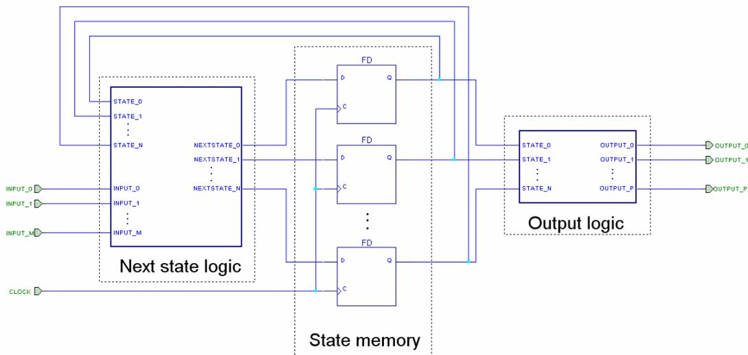
Figure 1: Block diagram for general state machine design
