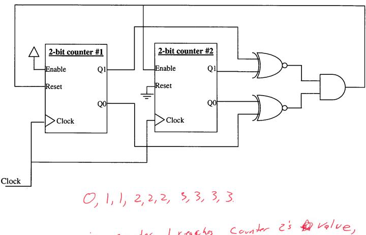
Every time counter I reaches counter 2's @ value, counter 1 is reset and counter 2 increments.
