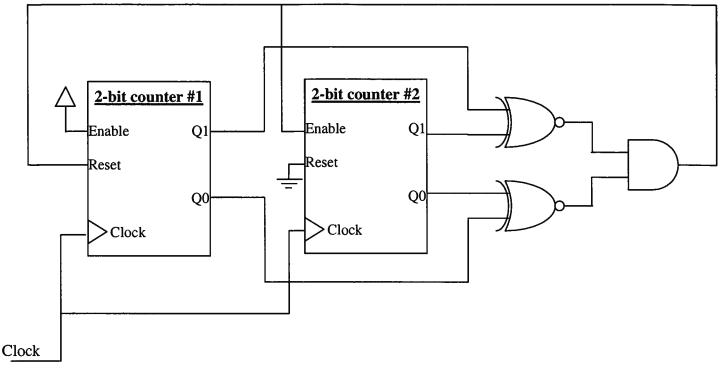
8) Consider the circuit diagram below where both counters are modulo counters and the resets are synchronous. Assuming both counters are initially zero, indicate the pattern that will appear out of counter #2. Write your answer using decimal numbers. So, for example, a possible (but wrong) answer would be "0, 1, 2, 1, 1, 3" which indicates that the output would be the pattern 012113012113012113 (etc.) repeating forever. Explain your answer. [9 points]
