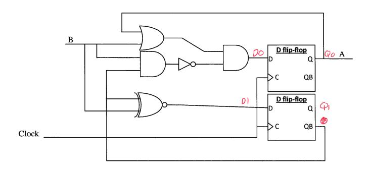
2) Draw the state transition diagram which is implemented by the above circuit. You should assume the initial state is when both flip-flops are "0". You should only include states that can be reached from the initial state. Clearly show your work. [12 points]
