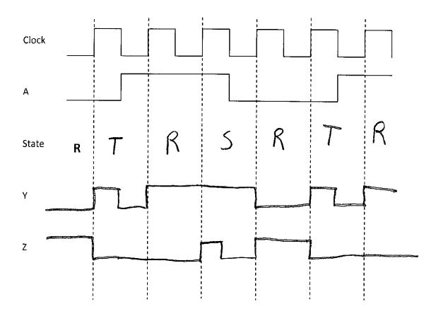
7. For this problem, assign state bits S[1:0] as 00 for state R, 01 for state S, and 10 for state T. <u>Using a K-map</u>, find the *minimal sum-of-products* for next state (NS[1:0]) and the outputs (Y and Z). You are to assume that any output not shown is zero and that you will never reach the state S[1:0]=11, so you don't care what happens in that case. You must show your work to get <u>any credit!</u> [10 points]
