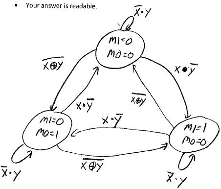
11. Using only 2 T-flip flops and no more than 2 standard gates (AND, NAND, NOT, XOR etc.) design a 2-bit up/down counter. The device is to count up when "up/down" is a 1 and down when "up/down" is a 0. C1 is the MSB. [6 points]
