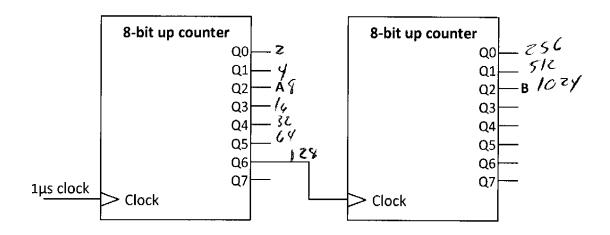
Frequency of A:  $\frac{1}{8 \mu s} = 125 \text{ KHz}$ Frequency of B:  $\frac{1}{1024 \mu s} = 977 \text{ Hz}$
