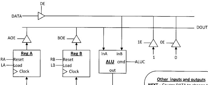
12. You are to design a state machine which causes the above datapath to find the average of 4 numbers (rounding down). When the START signal goes high, you are to begin to compute the average. Once done, the result should be placed on DOUT and the DONE signal should be set high. START will not go high again until after DONE is asserted.
