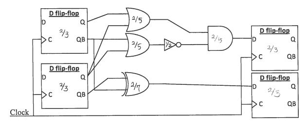
a. Assuming you want a reliable circuit, what is the highest value the flip-flop could have for a hold time? Show your work. [4 points]
