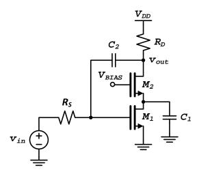
a) Draw the high-frequency small-signal model for the amplifier, including  $\mathcal{C}_1$  and  $\mathcal{C}_2.$
