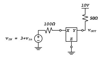
d) Draw the small-signal circuit for the circuit from part c). Derive an expression for the small-signal gain  $A_v=v_{out}/v_{in}$  and evaluate the gain at the DC operating point found in part c).
