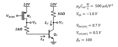
a) Assuming  $Q_1$  is kept in the forward-active region, find the numerical value of  $I_B$  required to support  $I_C = 1 \ mA$ .
