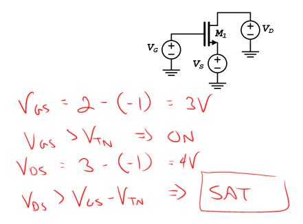
d) Identify the region of operation of  $M_1$  in the circuit below when  $V_G=3~V, V_D=5~V$ , and  $V_S=5~V$ . Assume  $V_{TP}=-1~V$  and ignore the body-effect on threshold voltage.
