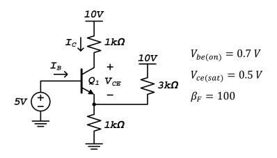
a) Substitute the simplified large-signal model for the BJT in the forward-active region using the constant-voltage source model for the base-emitter junction diode. Solve for the values of  $I_C$  and  $V_{CE}$ .
