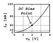
a) Derive an expression for the small-signal conductance  $i_m/v_m$ , linearized around a DC operating point defined by variables  $I_M$  and  $V_M$ .
