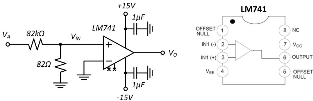
**Figure 3. Circuit for exercises L1.1 and pinout of LM741.**
