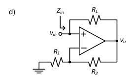
**P2.3** Derive an expression for the input impedance  $Z_{IN}$  of the non-inverting amplifier below. Assume a non-ideal opamp with finite gain  $A_0$  and input resistance  $R_{IN}$ . All other opamp parameters are ideal. Assume that  $R_{IN} \gg R_1$ ,  $R_2$  and use this to simplify your expression.
