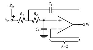
b) Given that  $\omega_n = \sqrt{R_1 R_2 C_1 C_2}$ , find an expression for d that fits the form of the 2<sup>nd</sup>-order expression from the Sallen & Key paper:
