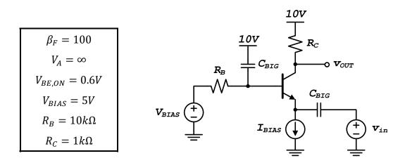
a) Draw the DC equivalent circuit. Calculate the value of  $I_{BIAS}$  that will bias the BJT in the FAR region, at the boundary between FAR and Saturation.
