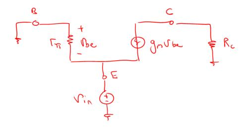
gn = 100 m T Tys = 1 Ks c) For this part, do NOT use the evaluated values of small signal elements found in part b). Derive an expression for the midband small-signal gain  $a_v = v_{out}/v_{in}$ . Leave this expression in terms of variable names  $(r_\pi, g_m,$  etc.). Assume  $V_A = \infty$ .
