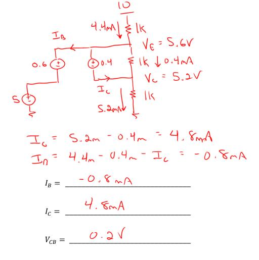
b) For this part, assume the BJT is in the FAR region. Use the simplified model for the BJT in FAR, using the constant-voltage-drop model for the E-B junction. Solve for the values of  $I_B$ ,  $I_C$ , and  $V_{CB}$  and enter them in the space below.
