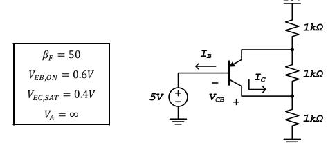
a) For this part, assume the BJT is in the Saturation region. Use the simplified model for the BJT in saturation, using the constant-voltage-drop model for the E-B junction and  $V_{EC,SAT}$ . Solve for the values of  $I_B$ ,  $I_C$ , and  $V_{CB}$  and enter them in the space below.
