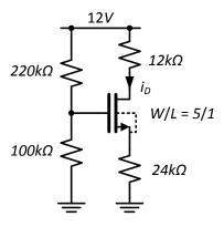
**P5.10** Choose values for  $R_1$  and  $R_2$  so that the DC bias current through the PMOS transistor is  $i_D=100\mu A$ , and the current through the biasing branch  $i_{R1}=i_{R2}=10\mu A$ . Assume  $V_{TP}=-1V$ ,  $\lambda=0$ , and  $\mu_p C_{ox}=K_p'=40\mu A/V^2$ .
