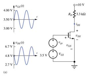
**P7.7** Calculate the DC bias current  $I_D$  for the circuit on the right assuming  $K_n = 250 \mu A/V^2$ ,  $V_{tn} = 1V$ , and  $\lambda = 0$ . Calculate the new value of  $I_D$  and the percentage change in  $I_D$  resulting from a 5% increase in  $K_n$  ( $K_n = 262.5 \mu A/V^2$ ). Calculate the new value of  $I_D$  and the percentage change in  $I_D$  resulting from a 5% decrease in  $V_{tn}$  ( $V_{tn} = 0.95V$ ).
