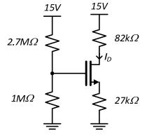
P7.8 Calculate the DC bias current  $I_D$  for the circuit below assuming  $K_p=100\mu A/V^2$ ,  $V_{tp}=-1V$ , and  $\lambda=0$ . Calculate the new value of  $I_D$  and the percentage change in  $I_D$  resulting from a 5% increase in  $K_p$  ( $K_p=105\mu A/V^2$ ). Calculate the new value of  $I_D$  and the percentage change in  $I_D$  resulting from a 5% decrease in  $V_{tp}$  ( $V_{tp}=-0.95V$ ).
