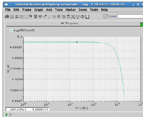
Here again we see that the non-inverting amp is giving us a gain of about  $A_v = 5$ . Since this is not an ideal op-amp we can see it starting to cut-off at higher frequencies. If you run a wider frequency simulation, you will see where the amplifier cuts off.
