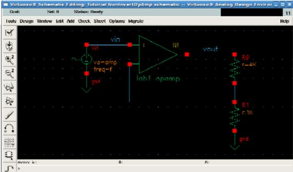
$$A_v = 1 + \frac{R_2}{R_1} \quad \begin{array}{l} R_2 = 4k\Omega \\ R_1 = 1k\Omega \end{array}$$
