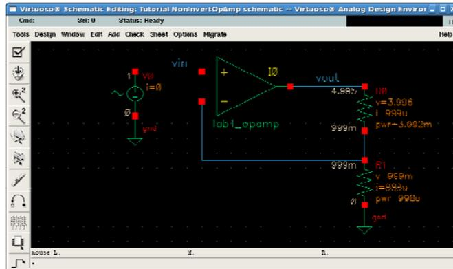
As expected, the op-amp shows roughly equal DC voltage at its terminals with no DC current going to either one. From the non-inverting architecture we also see that we obtain a gain of roughly  $A_v = 5$  V/V which is expected from the aforementioned equation.
