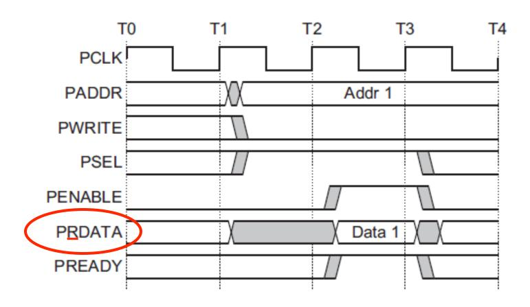
The key thing here is that each slave device has its own read data (PRDATA) bus!
