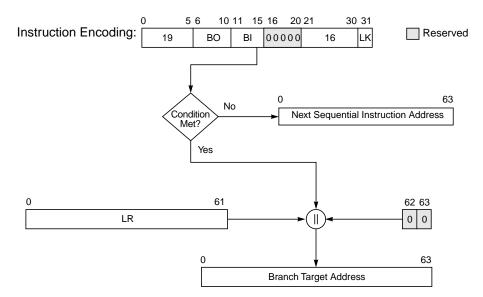
Figure 4-10. Branch Conditional to Link Register Addressing
