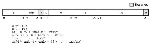
The contents of  $\mathbf{r}A$  are compared with the contents of  $\mathbf{r}B$ , treating the operands as unsigned integers. The result of the comparison is placed into CR field  $\mathbf{crf}D$ .
