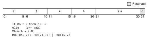
EA is the sum  $(\mathbf{rA}|0) + (\mathbf{rB})$ . The contents of the low-order eight bits of  $\mathbf{rS}$  are stored into bits 0–7 of the half word in memory addressed by EA. The contents of the subsequent low-order eight bits of  $\mathbf{rS}$  are stored into bits 8–15 of the half word in memory addressed by EA.
