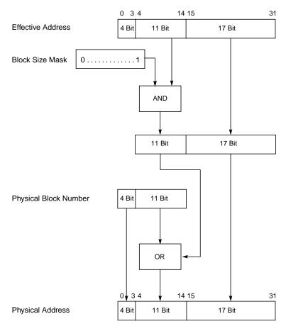
Figure 7-10. Block Physical Address Generation
