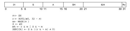
The contents of **rS** are shifted right the number of bits specified by operand SH. Bits shifted out of position 31 are lost. The shifted value is sign-extended before being placed in **rA**. The 32-bit result is placed into **rA**. XER[CA] is set if **rS** contains a negative number and any 1 bits are shifted out of position 31; otherwise XER[CA] is cleared. A shift amount of zero causes XER[CA] to be cleared.
