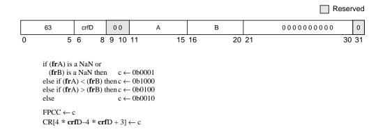
The floating-point operand in register **fr**A is compared to the floating-point operand in register **fr**B. The result of the compare is placed into CR field **crf**D and the FPCC.
