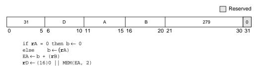
EA is the sum  $(\mathbf{r}A|0) + (\mathbf{r}B)$ . The half word in memory addressed by EA is loaded into the low-order 16 bits of  $\mathbf{r}D$ . The remaining bits in  $\mathbf{r}D$  are cleared.
