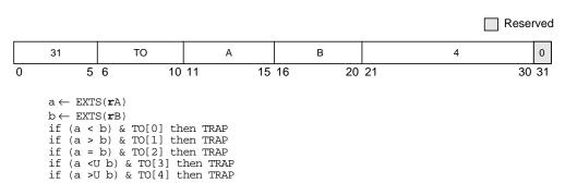
The contents of **r**A are compared with the contents of **r**B. If any bit in the TO field is set and its corresponding condition is met by the result of the comparison, then the system trap handler is invoked.
