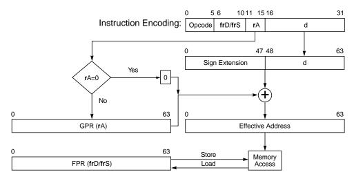
Figure 4-4. Register Indirect with Immediate Index Addressing for Floating-Point Loads/Stores
