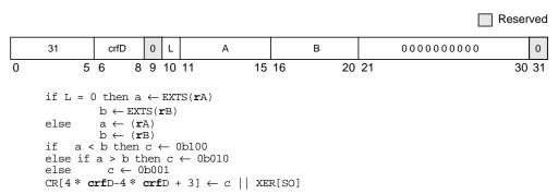
The contents of  $\mathbf{r}A$  are compared with the contents of  $\mathbf{r}B$ , treating the operands as signed integers. The result of the comparison is placed into CR field  $\mathbf{crf}D$ .
