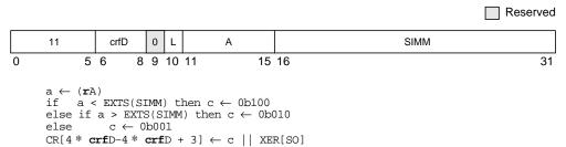
The contents of  $\mathbf{r}A$  are compared with the sign-extended value of the SIMM field, treating the operands as signed integers. The result of the comparison is placed into CR field  $\mathbf{crf}D$ .
