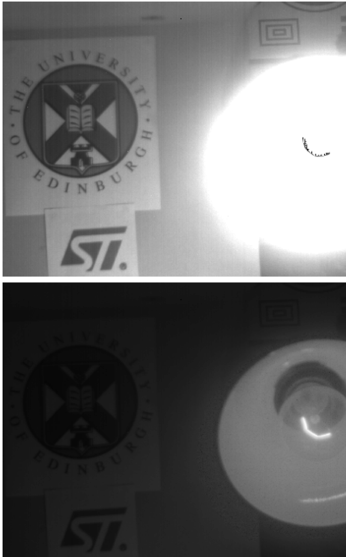
Fig. 23. Top: Linear image (including CDS breakdown). Bottom: Combined linear logarithmic image.
