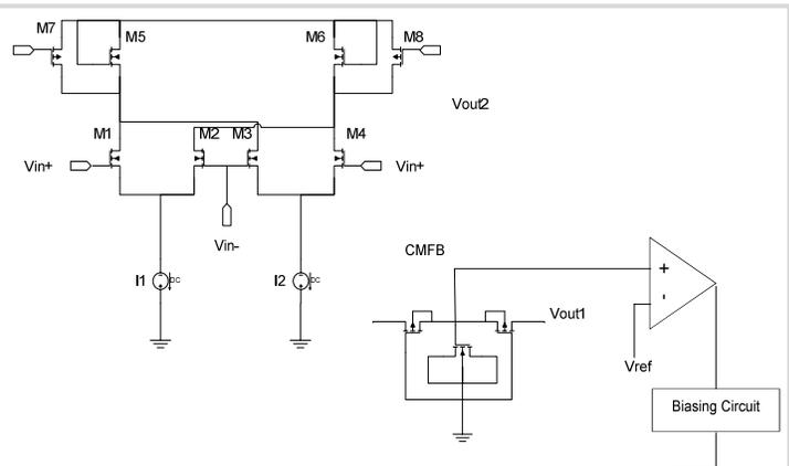
Figure 2A: Schematic of VGA
