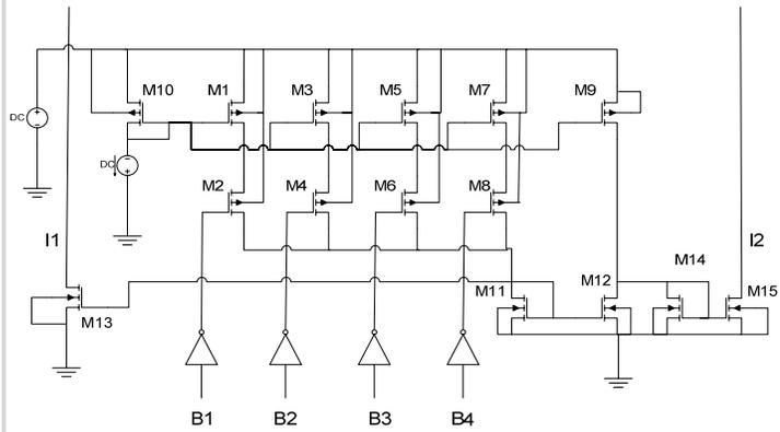
Figure 3: Schematic of Digital Control Circuit
