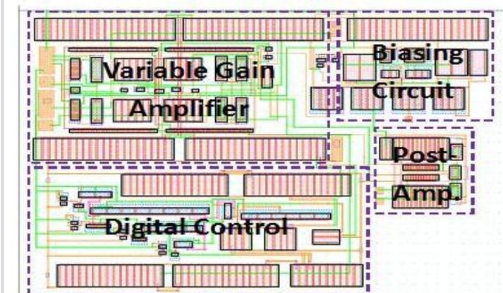
Figure 5: Layout in Cadence(DRC and LVS clean )
