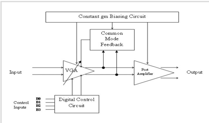
Figure 1: Block diagram of proposed VGA cell
