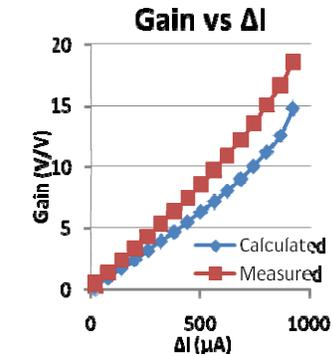
Figure 6A: Voltage gain vs. Control current
