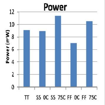
Figure 6B: Power consumption with different corners
