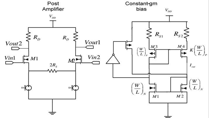
Figure 4A: Schematic of Post-Amp
