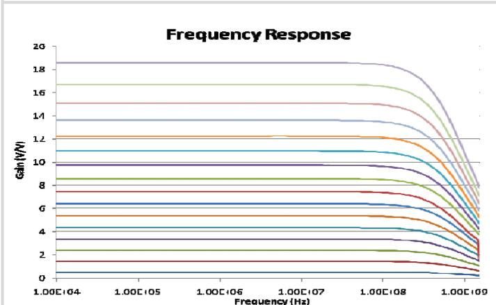
Figure 7: Frequency response of different gains of VGA cell in magnitude
