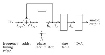
(a) (2 pts) Suppose FTV = 4,  $f_s = 10$ MHz,  $B_{FTV} = 12$ , and the sine table contains 256 values denoted as  $x(0), x(1), \dots, x(255)$ . Assume the system is initialized to zero. Please write down the first 10 values coming out of the sine table, each upon a clock tick.
