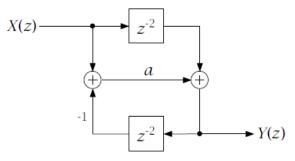
c. Write a function, short trans (short x, short \*w) which takes a single input x, and returns the y value. Assume a=2 and that the array w is used for as many z<sup>-1</sup> blocks and is of any fixed size you find useful. You may assume all inputs are in 16-bit Q15 and no overflow occurs. [8 points]
