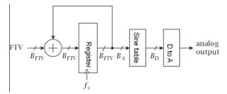
3) *JoeBlow Audio* has hired you to build them a digital device which outputs a sine 500Hz sine wave which has a 2 Volt amplitude (it ranges from -2 to 2 Volts). They want the sine wave to never be more than 5mV different from an ideal (real number) sine wave with the same frequency and amplitude. You may assume you can get an output of exactly 500Hz.
