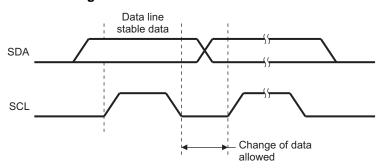
Figure 5. Bit Transfer on the I2C-Bus
