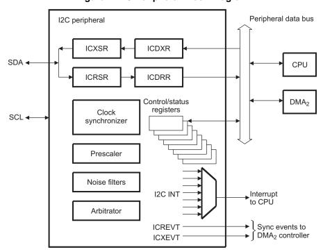
Figure 1. I2C Peripheral Block Diagram
