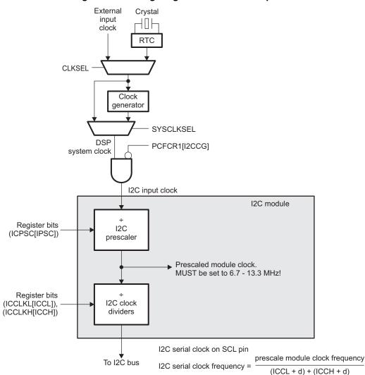
Figure 3. Clocking Diagram for the I2C Peripheral
