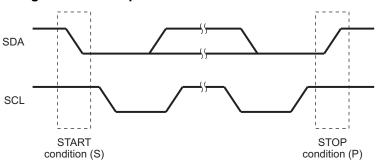
Figure 6. I2C Peripheral START and STOP Conditions
