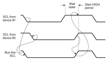
Figure 4. Synchronization of Two I2C Clock Generators
