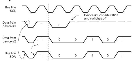
Figure 12. Arbitration Procedure Between Two Master-Transmitters
