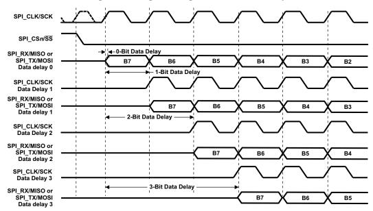
Figure 8. Range of Programmable Data Delay
