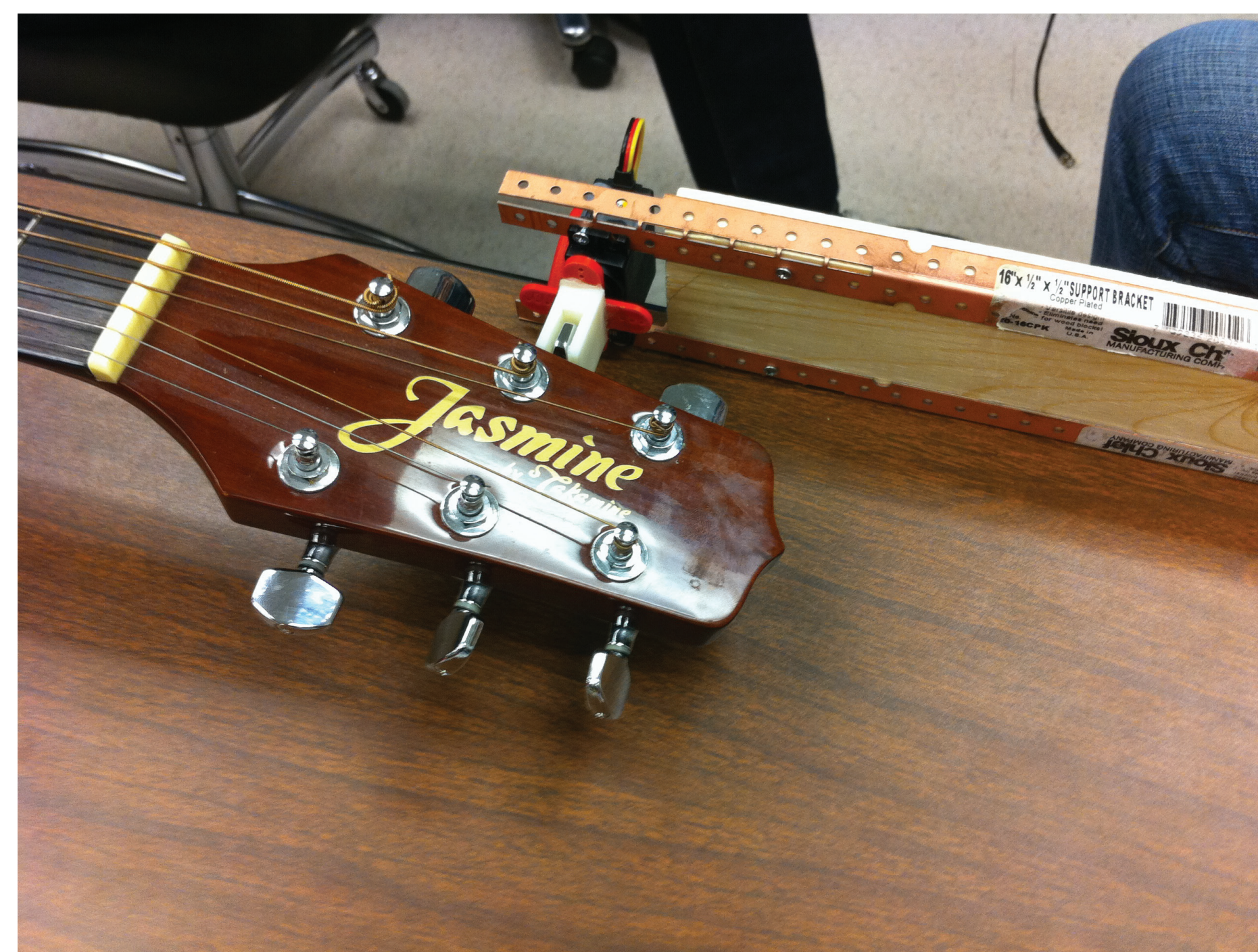
Figure 4: Prototype system tuning 'A' string (110 Hz)
