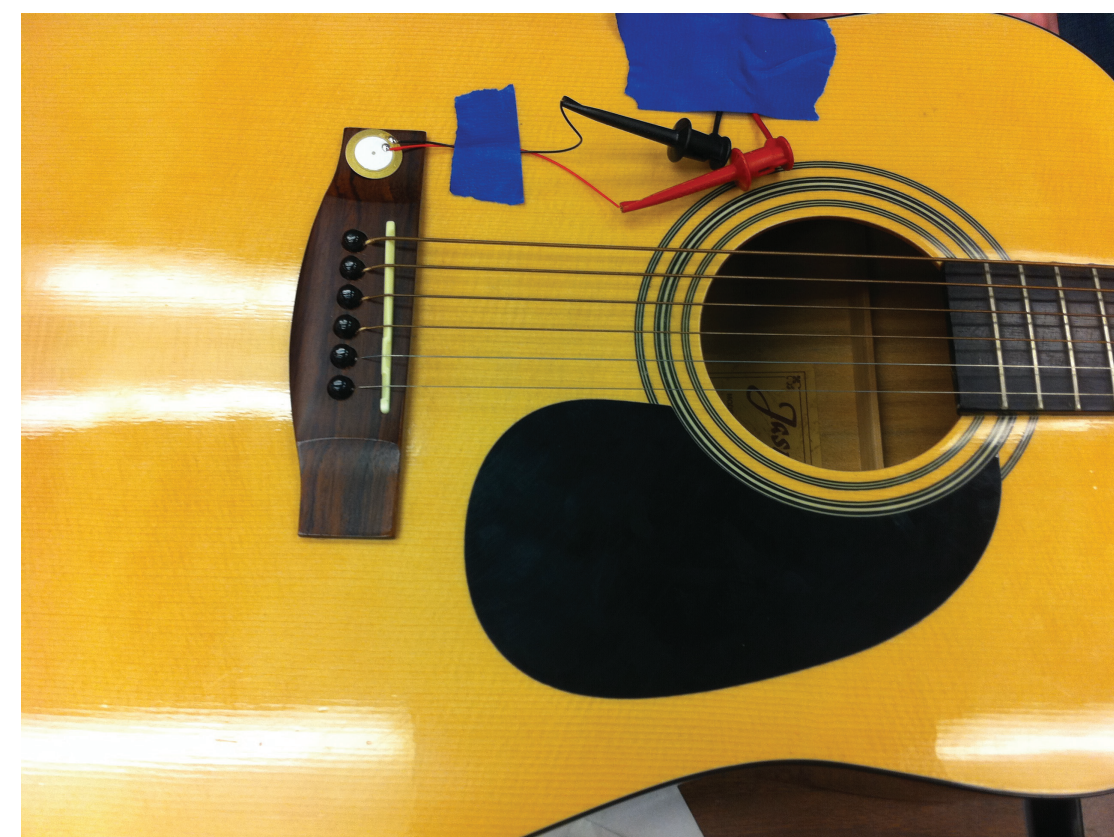
Figure 2: Placement of sensor on guitar, tape removed
