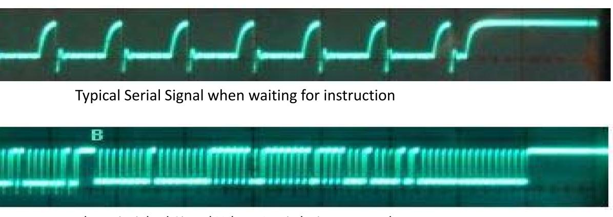
The Mimicked Signal When A, B is being pressed
