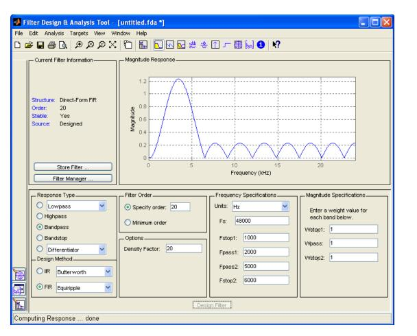
The filter coefficients for the equalizer were generated with MATLAB's fdatool. Fdatool allows a filter designer to select the type of filter (high-pass, low-pass, band-pass, or bandstop) type of impulse response (FIR or IIR), type of design method (Butterworth, Equiripple, etc), cutoff frequencies, gain, and order.
