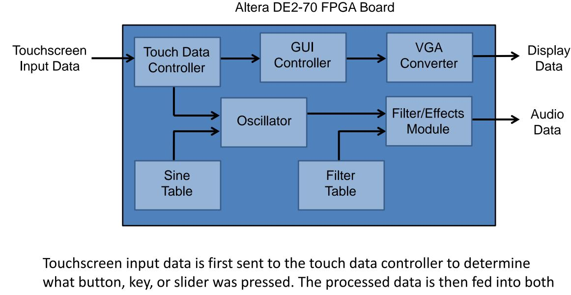
the visual and audio data paths. The visual data path updates the LCD display, and the audio path generates the selected waveform / frequency and applies any selected filters.
