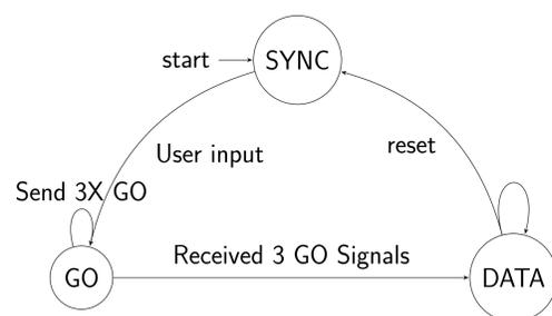
Figure: The state diagram for the encoder and decoder.
