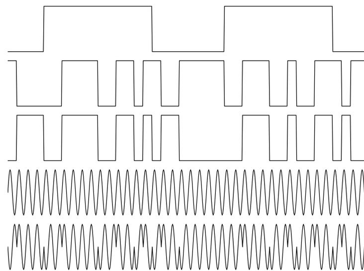
Figure: Diagram of various signals used to encode data using a spread spectrum technique.
