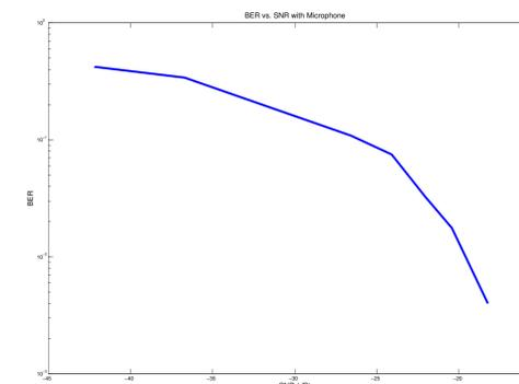
Our team performed an analysis of bit error rate using a prototype system consisting of a microphone/pre-amp and speakers as the input and output to a transmitter/receiver pair. During the test, the music we used as input to the transmitter was the Beatle's "Ticket to Ride".
