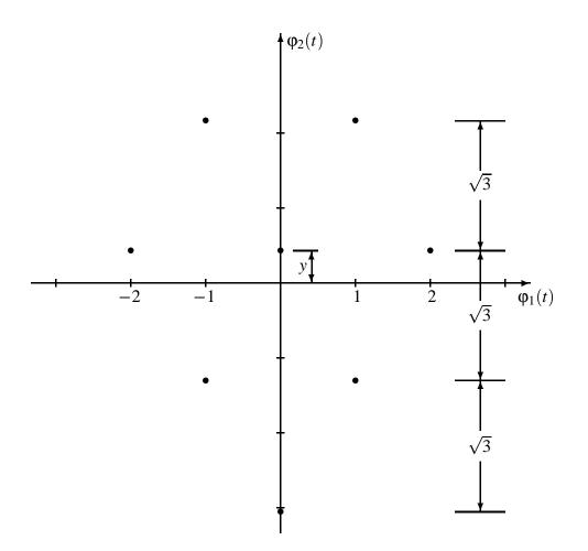
3. A modulator uses two orthonormal signals ( $\phi_1(t)$  and  $\phi_2(t)$ ) to transmit 3 bits of information (8 possible equally likely signals) over an additive white Gaussian noise channel with power spectral density  $N_0/2$ . The signals are given as
