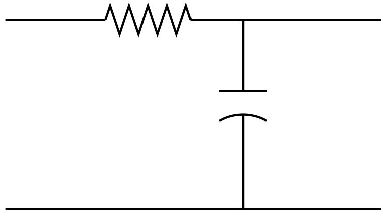
$$\begin{aligned} h(t) &= \frac{1}{RC} e^{-t/RC} u(t) \\ &= \alpha e^{-\alpha t} u(t), \quad \alpha = 1/RC \\ \|h\| &= \int_{-\infty}^{\infty} h^2(t) dt = \int_0^{\infty} \alpha^2 e^{-2\alpha t} dt \\ &= \frac{\alpha^2}{-2\alpha} e^{-2\alpha t} \Big|_0^{\infty} = \frac{\alpha}{2} \end{aligned}$$
