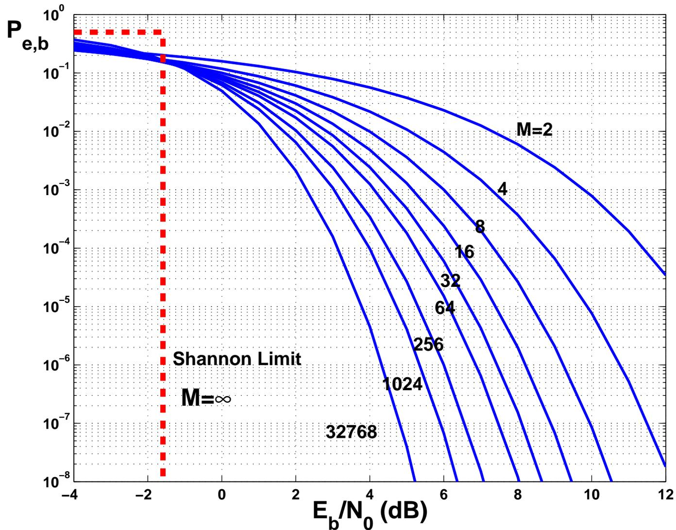
Figure 45: Bit Error Probability for Coherent Demodulation of Orthogonal Signals
