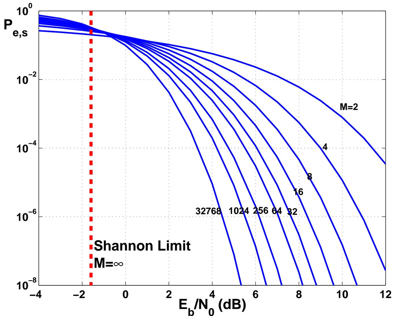
Figure 44: Symbol Error Probability for Coherent Demodulation of Orthogonal Signals
