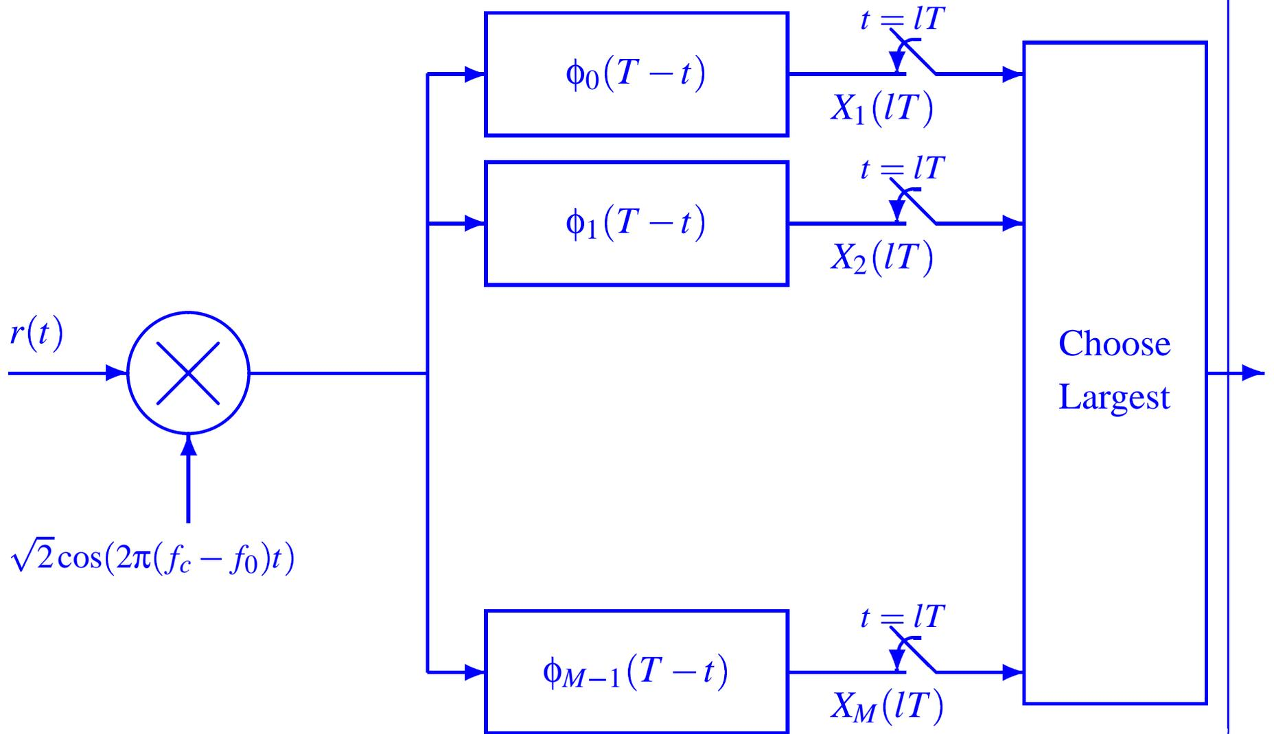
$\phi_m(T - t)$  is the impulse response of the  $m$ -th matched filter. The output of these filters (assuming that the  $i_l$ -th orthogonal signal is transmitted is) given by
