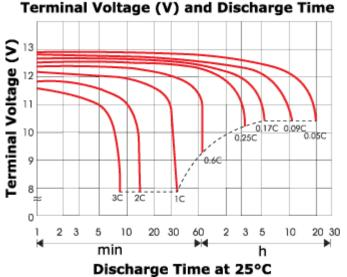
b) *About* how long could a 750mAh battery of the chemistry to the left drive a  $50\Omega$  load that requires at least 11 Volts? **[6]**
