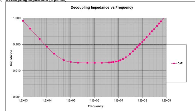
The above graph shows the frequency vs. impedance for a given capacitor. Redraw the graph showing the same information but if we instead put used 2 new capacitors (in parallel) which each had the same ESR and ESL but five times the capacitance.
