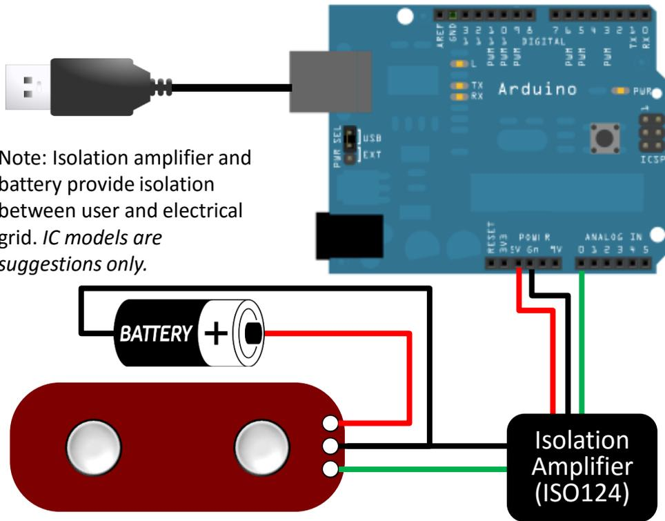
*(Note: Arduino and batteries not included. Arduino setup is only an example; sensor will work with numerous other devices.)*
