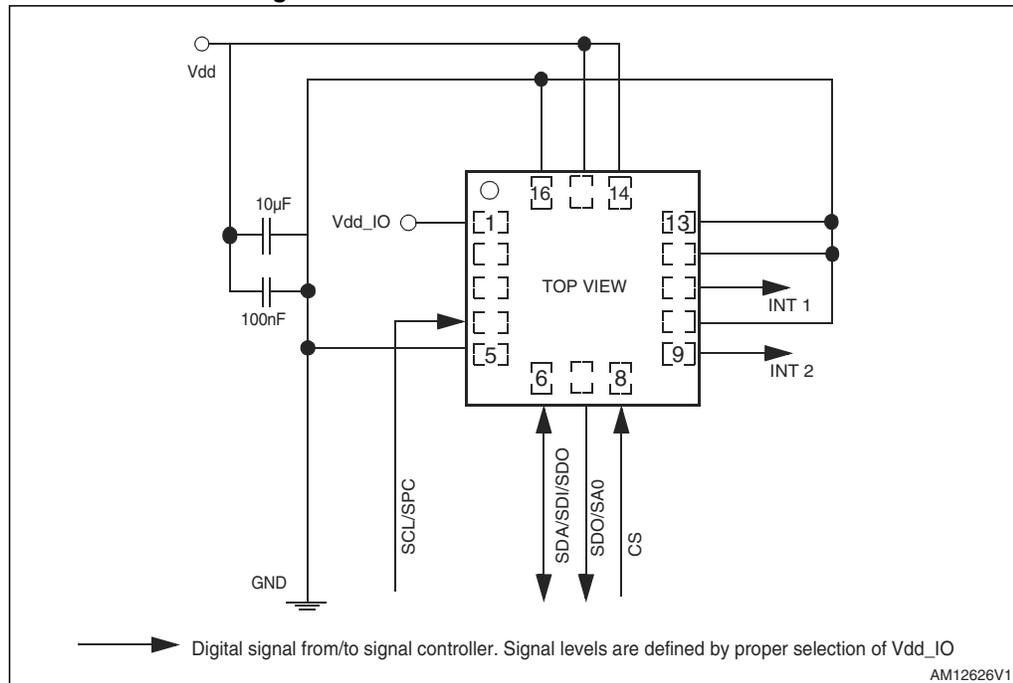
The device core is supplied through the Vdd line while the I/O pads are supplied through the Vdd\_IO line. Power supply decoupling capacitors (100 nF ceramic, 10 µF aluminum) should be placed as near as possible to pin 14 of the device (common design practice).
