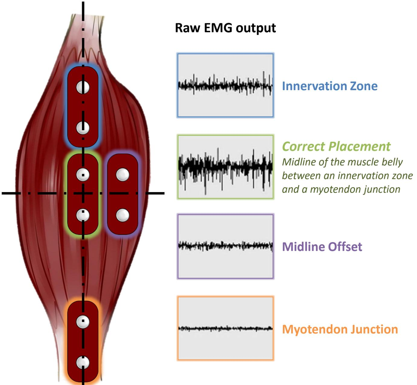
Position and orientation of the muscle sensor electrodes has a vast effect on the strength of the signal. The electrodes should be placed in the middle of the muscle body and should be aligned with the orientation of the muscle fibers. Placing the sensor in other locations will reduce the strength and quality of the sensor's signal due to a reduction of the number of motor units measured and interference attributed to crosstalk.
