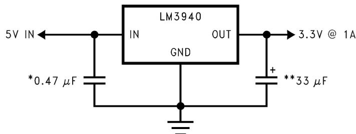
\*Required if regulator is located more than 1 inch from the power supply filter capacitor or if battery power is used.
