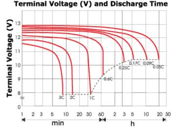
b) *About* how long could a 750mAh battery of the chemistry to the left drive a  $50\Omega$  load that requires at least 11 Volts? **[6]**
