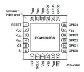
**Part 2** Write the initialization function for the PCA9502 GPIO expander. This should include Arduino pin initialization and creating an SPI configuration. Note you must reset the device before communicating to it. You also will want to have the function "measure\_speed" called when there is a change in one of the signals coming from the wheel. Fill in the blank for the SPISettings. **[10 points]**
