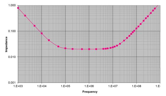
6. The above graph shows the frequency vs. impedance for a given non-ideal capacitor. Redraw the graph showing the same information if an ideal capacitor with the same capacitance was placed in parallel with the non-ideal capacitor. **[5 points]**
