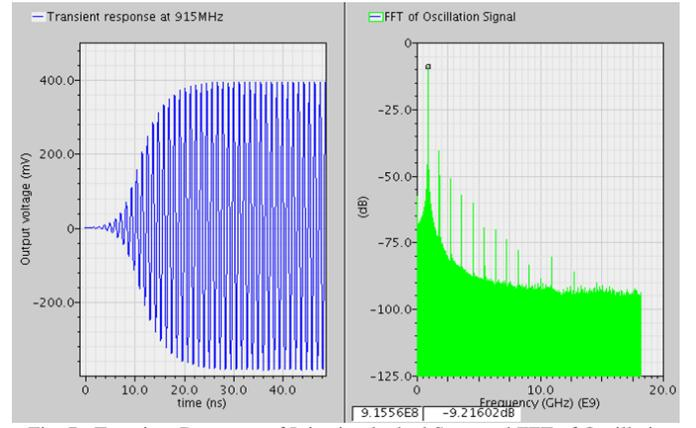
Fig. 7. Transient Response of Injection locked State and FFT of Oscillation Signal
