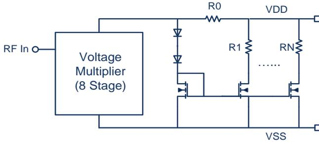
Fig. 3. 8 Stage Voltage Multiplier and Limiter
