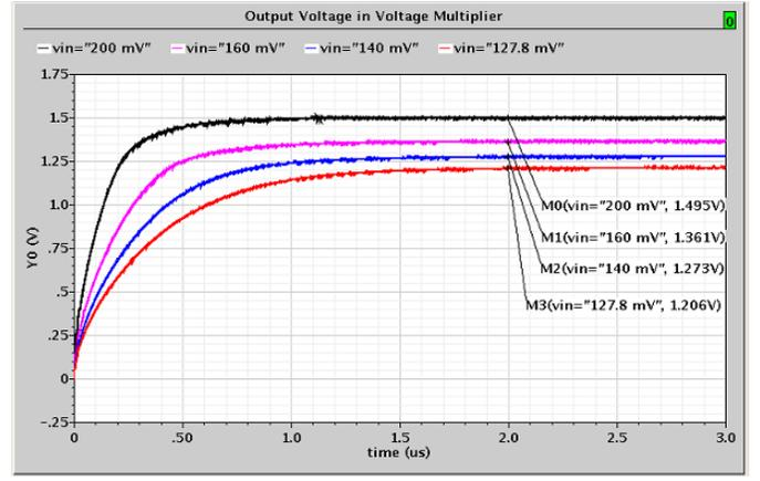
Fig. 4. 8 Stage Voltage Multiplier and Limiter
