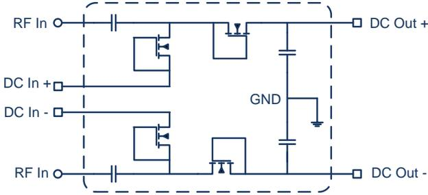
Fig. 2. Single Stage of Full-Wave Rectifier
