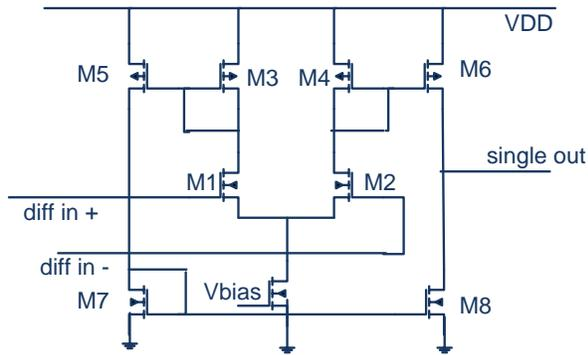
Fig. 10. Two Stage OP Amp with Single Ended Output
