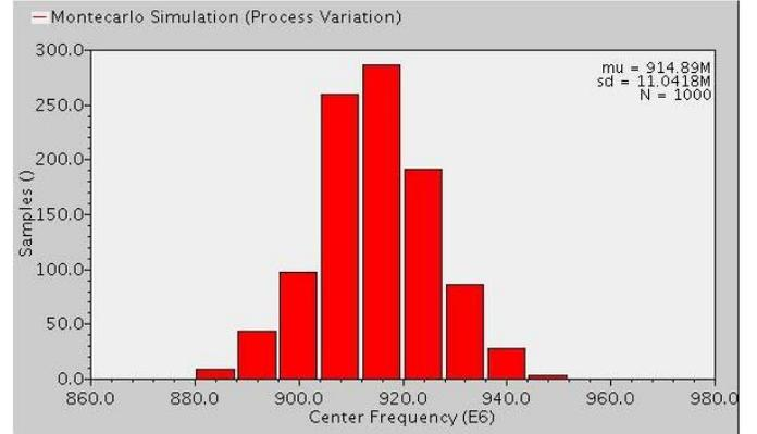
Fig. 8 Device working range over process variation with 140mV incident signal
