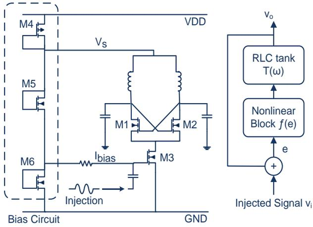
Fig. 5. Schematic and Block Model of Injection Locked Oscillator
