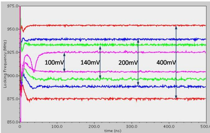
Fig. 6. Lock-in Range Limit for Different Incident Signal Voltages (100 to 400mV)
