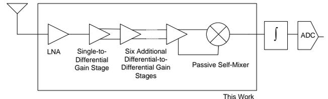
Figure 1: Block Diagram of UWB Receiver
