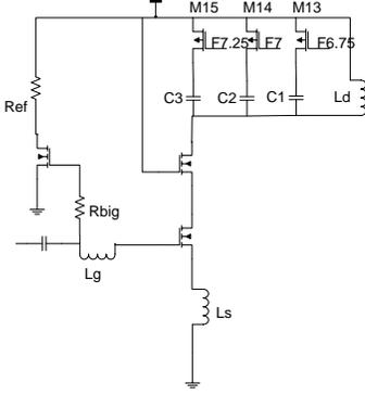
**Figure 2: Cascoded Common Source LNA with Inductive Degeneration**
