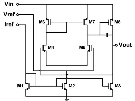
Fig.2 Schematic of Low drop out voltage regulator.
