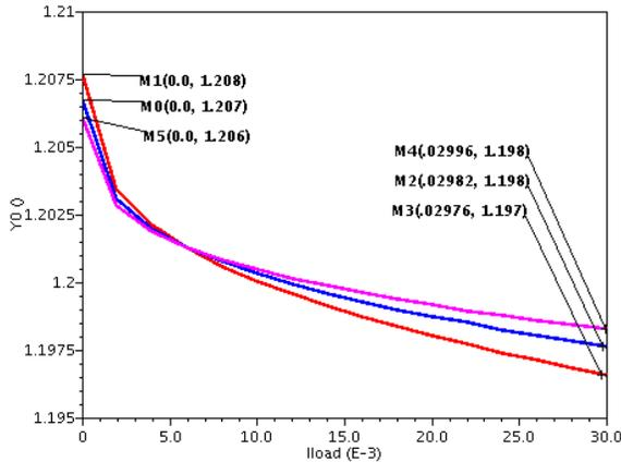
Fig.6. Simulated load regulation over an output current range of 30mA, showing a change in output voltage of only 1.1 mV.
