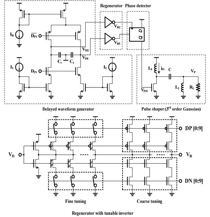
Fig.3. Circuit schematic of pulse generator
