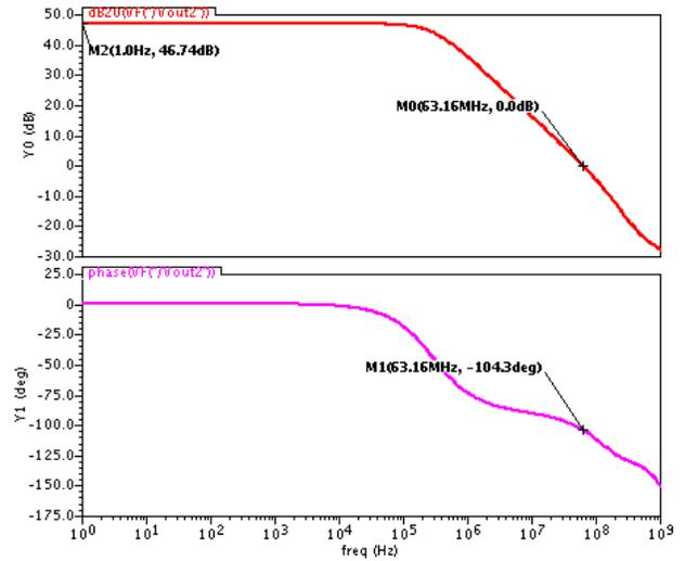
Fig.8. Open Loop Gain and Phase plot
