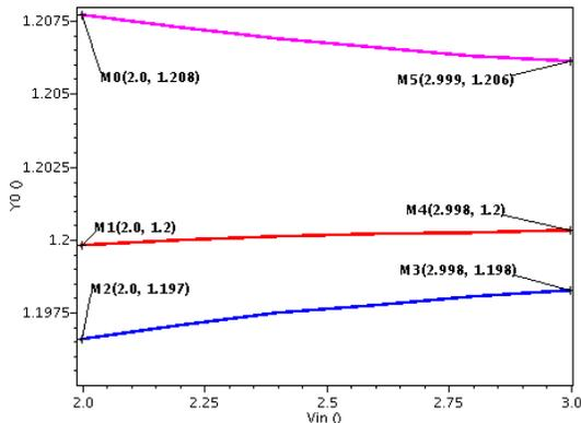
Fig.7. Simulated line regulation over a supply voltage variation of  $\pm 20\%$  from nominal value, showing a change in output voltage of 0.1 mV.
