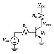
**Problem 1.3:** Use the circuit on the right for this problem. Assuming the transistor is biased in the forward active region, calculate the numerical value for small signal gain given  $V_A = 35V$ . Assume room temperature. This is what is referred to as the "intrinsic gain" of the device.
