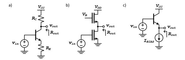
**Problem 1.2:** Use the circuit on the right for this problem. Include base width modulation in your calculations. Assume  $\beta_F$  = 120,  $V_A$  = 35V,  $V_{CE(sat)}$  = 0.3V, and  $V_{BE}$  = 0.7V when  $Q_1$  is in the forward active region.
