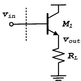
$$V_{out} / V_{in=0} = (i_B + i_C + i_{RL}) \cdot \left( \frac{1}{g_m} \parallel R_L \parallel \frac{1}{j\omega C_L} \right)$$
