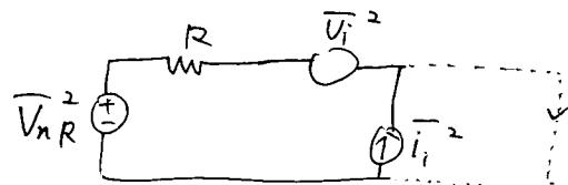
$$F = \frac{\frac{\overline{V_n R}^2 + \overline{V_i}^2}{R^2} + \overline{i_i}^2}{\frac{\overline{V_n R}^2}{R^2}} = \frac{\overline{V_n R}^2 + \overline{V_i}^2 + \overline{i_i}^2 R^2}{\overline{V_n R}^2}$$
