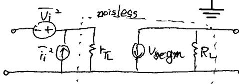
To get  $\overline{V_i^2}$ , short both inputs (noisy and noiseless)
