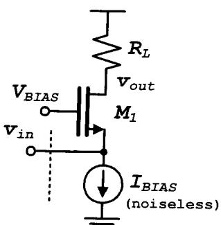
$$\overline{V_{out}^2} = [4KT \delta g_m + 4KT \frac{1}{R_L}] R_L$$
