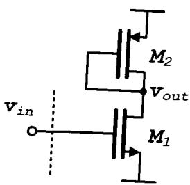
$$\overline{V_{out}^2} = 4KT(\delta_n g_{m1} + f_p g_{m2}) \left( \frac{1}{g_{m2}} \right)^2 \Delta f$$
